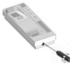
To open the telephone, insert a plain screwdriver into the slots and gently lever as shown in the drawing.
